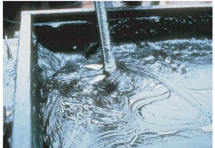
A series of pump tests were conducted from October to December 2004 to measure the suction capability of the Salarollpump with high viscous oil.
