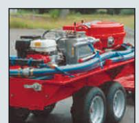
The ease of transporting the system is further enhanced by handles that attach to both the pump and power pack for lifting in difficult terrain or by wheeling it as a wheel barrow. An all terrain vehicle or band driven vehicle attached to a trailer is available to transport the pump and power pack to the impacted area. The trailer can also be used for transporting smaller amounts of oil in sacks or barrels to the collecting area.
